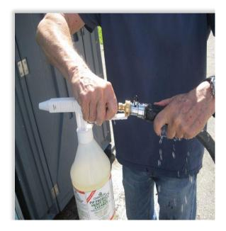
Inserting the quick disconnect into the foaming head
